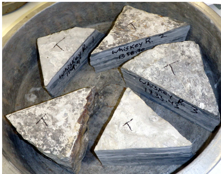
Whiskey River samples before 30 freeze-thaw cycles.
