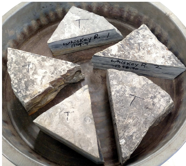
Whiskey River samples after 30 freeze-thaw cycles.
