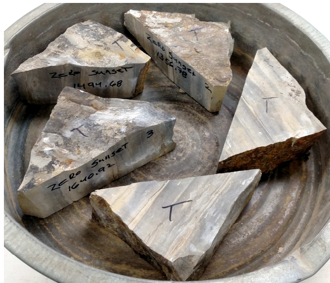
Zero Sunset samples after 30 freeze-thaw cycles.
