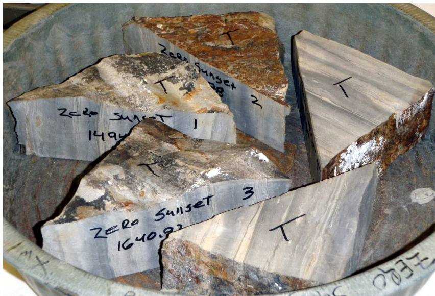
Zero Sunset samples before 30 freeze-thaw cycles.
