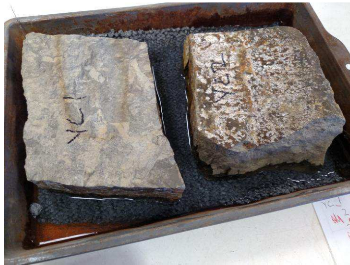
Yellow crusher samples YC1 and YC2 following freeze-thaw.
