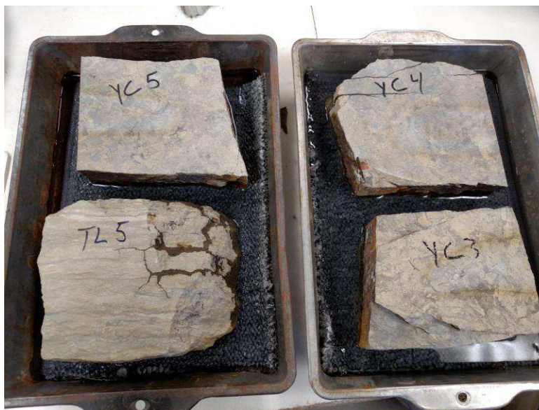
Yellow crusher samples YC3, YC4 and YC5 following freeze-thaw.
